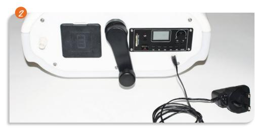
Attach the mains power lead to the power connector located at the top of the model (underneath the MP3 Player). Plug into power source
